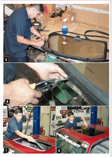
5 Work your way around the sunroof frame, pressing the weatherstripping firmly onto the frame rail.
