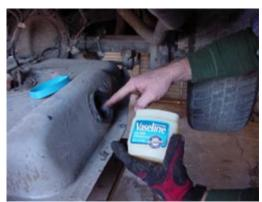
17. Put some petroleum jelly on the filler neck seal to help the filler neck slide into place.
