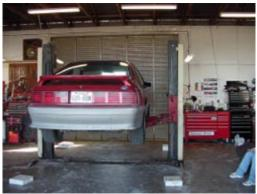
1. Safely lift vehicle and support it before doing any work, be sure to read over your instructions on the work being preformed.
