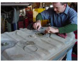
15. Install the new "O-ring" seal and reinstall the fuel pump assembly.
