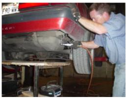
2. Using a 1/4" drive ratchet and an 8mm socket, disconnect the filler neck strap.
