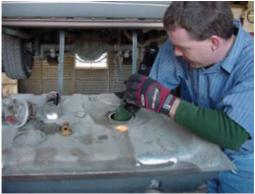
13. Before you put the assembly back in the tank be sure to clean out any debris that may cause premature pump failure.
