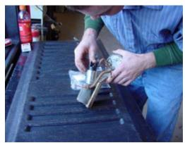
11. After extracting the old pump out of the assembly you may now install the new pump.
