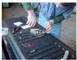
12. Reconnect the electrical per the instructions that came with your pump. Double check all your work as you will not want to have to remove the tank again just for a loose connection.
