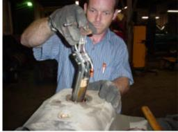
10. Carefully turn and maneuver the pump assembly out of the tank. With the pump assembly out, you can now service the pump.
