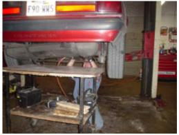
3. Place a table or jack under the tank to catch it when you undo the tank straps. The 2 strap bolts are released with a 13mm socket.
