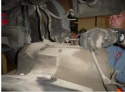
6. If you have the plastic "inverted" clip on your return line you can release it with a pair of needle nosed pliers.
