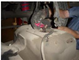
5. Then with the fuel clip releasing tool, undo the "return" line.
