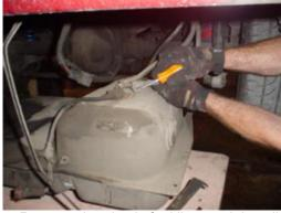
4. Remove the plastic fuel line retaining clip holding the "feed" line on.
