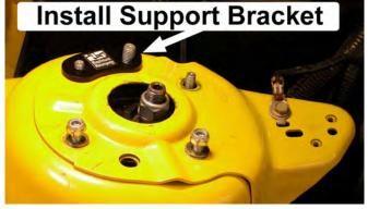
28. Place one of the provided large G8 washers on to the Caster Plate Stud, followed by one of the provided 10mm Nylock nuts and thread it on until the tip of the bolt touches the Nylock portion of the nut.
