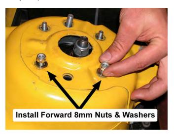
27. Place the passenger side Support Bracket onto the protruding studs, as shown in the photo. The Support Bracket should be oriented towards the outboard side of the vehicle.
