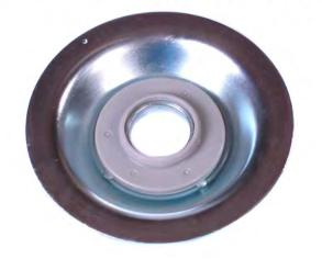
NOTE: The Bearing Plates are not side specific, but they must be correctly oriented during installation in order to properly function. For correct orientation, the circular notch on the Bearing Plate must face towards the outboard side of the vehicle and the spherical bearing must be below the Bearing Plate.
