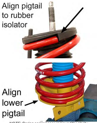
NOTE: Spring compressor removed for clarity.
