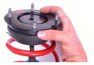
NOTE: Spring compressor removed for clarity.
