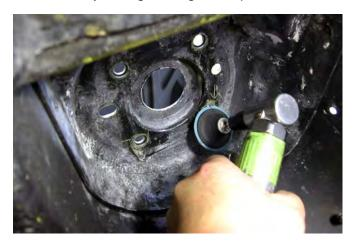
NOTE: Do not tighten the MM Caster/Camber Plate mounting nuts until instructed to do so. Thread the nuts on by hand until the tip of the bolts touch the Nylock portion of the nut.
