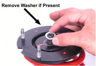
15. Remove the upper strut mount assembly from the strut shaft.
