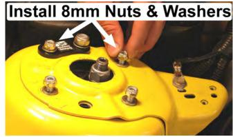
30. Reach through the hole in the top of the strut tower, and pull on the rubber band attached in Step 4 until it breaks. Completely remove the rubber band. Snug all five nuts on the MM Caster/Camber Plate.
