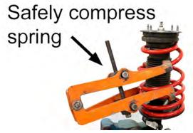
14. Remove the upper strut-retaining nut, and washer if present.
