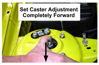
35. Next, center the strut shaft in the strut tower opening side to side. Once centered, torque the four 8mm Nylock nuts to 20 lb-ft.
