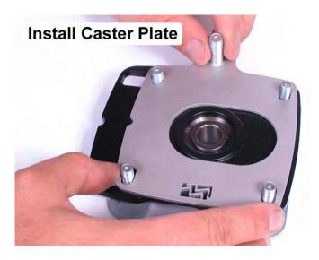
Large Radius Towards Spherical Bearing
