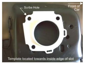
13. Slide the Ford top plate to align the holes with the outer edge of the factory slots and scribe a second hole.
