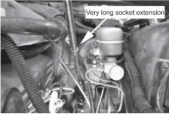
Disconnect the steering shaft from the steering rack input shaft.
