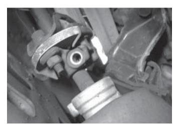
Most aftermarket steering shafts are secured to the input shaft with a setscrew and jam nut.
