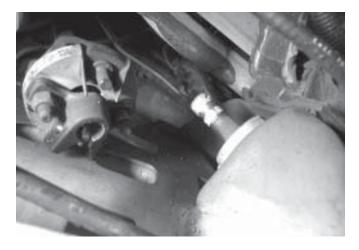
Stock steering shafts are secured to the input shaft of the steering rack with a pinch-bolt.
