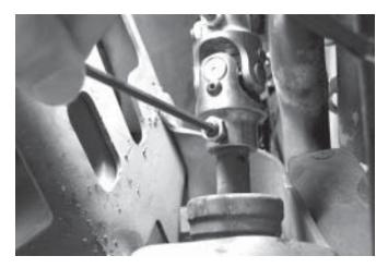
5. Rotate the steering wheel so that the front tires are steered straight ahead.
