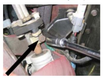
3. Remove the stock steering shaft upper pinch bolt located underneath the dash, where the steering shaft connects to the upper U-joint.
