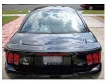
▲ Here is the rear section of our upgraded Pony. Fitment in the OEM location is another reason why we selected the S281 tail instead of others, which require drilling new or additional holes in the decklid for installation. This wing provides a clean, low line and when properly installed, looks like it belongs on this car
