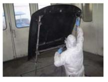
▲ The Mach 2 ram-air hood is attached to a painter's rack that allows Danny to cover every inch of both sides with fresh black paint. The hood remains on this rack for clearcoat and to dry before being moved to the FAB installation department.
