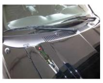
▲ A new cowl definitely cleans up the 'Stang's nose area. You don't realize how bad a cracked piece looks until it's replaced with a new one.
