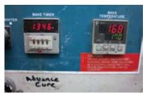
▲ Our web-watchers may have seen this image already, as it was used in your tech editor's blog section to highlight this report. All of the parts are baked in this spray booth/oven at FAB before any chemicals or finishes are applied. Baking the parts (170 degrees for 20 minutes) helps lift oils and contaminants from the material, making it "porous" and better able to accept sealer and paint.
