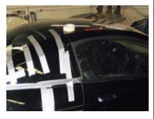
▲ Drying time for the 3M bonding agent is 24 hours. All of the tape is necessary for holding our scoops in place while the glue sets up.
