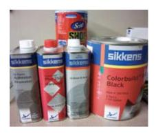
▲ Things start to get more serious in Stage 2 of the renovation effort. This suite of materials (adhesion promoter, hardener, Elast-O-Actif, and primer) is used once all the parts are clean and ready for paint. The Elast-O-Actif is designed to help paint cover and adhere to urethane-type pieces that are flexible, like our new scoops and rear spoiler, and especially on Mustangs' bumper covers.
