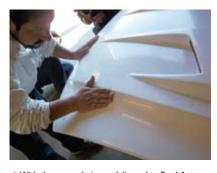
▲ With the car and pieces delivered to Ford Auto Body, Danny starts the makeover by assessing each of the pieces being installed. A body man's fingers actually are his most-important tools, as they transmit the presence of imperfections in a Mustang's body panels as well as in replacement parts. The Mach 2 hood and other parts passed Danny's inspection with flying colors. The entire set is of excellent quality and should require only standard prep work before they are painted.
