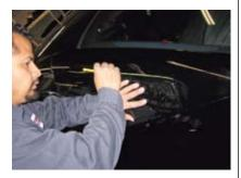
▲ All of the scoops and rear spoiler were pre-fit before they were painted and didn't require any trimming or modification. When applying the painted scoops, Hector uses yellow grease pencil to index exactly where the parts are placed over the rearquarter windows and lower quarter panel.
