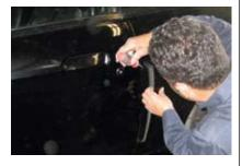
▲The 'Stang's original sidescoops are removed by simply prying them away from the rear quarterpanels using a small screwdriver and a light touch.
