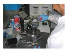
▲ Mixing paint is literally at a scientific level nowadays, which ensures color-matching is spot-on. Danny references a guide that details exactly how much paint, hardener, and such must be added to the mixture to cover various areas or parts.
